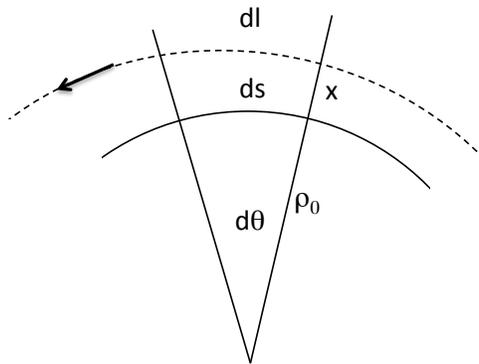
Figure 1: Curvilinear coordinate system. The integrated path length for the part of the trajectory at  $\rho > \rho_0$  is greater than the length of the path for  $\rho < \rho_0$ .
