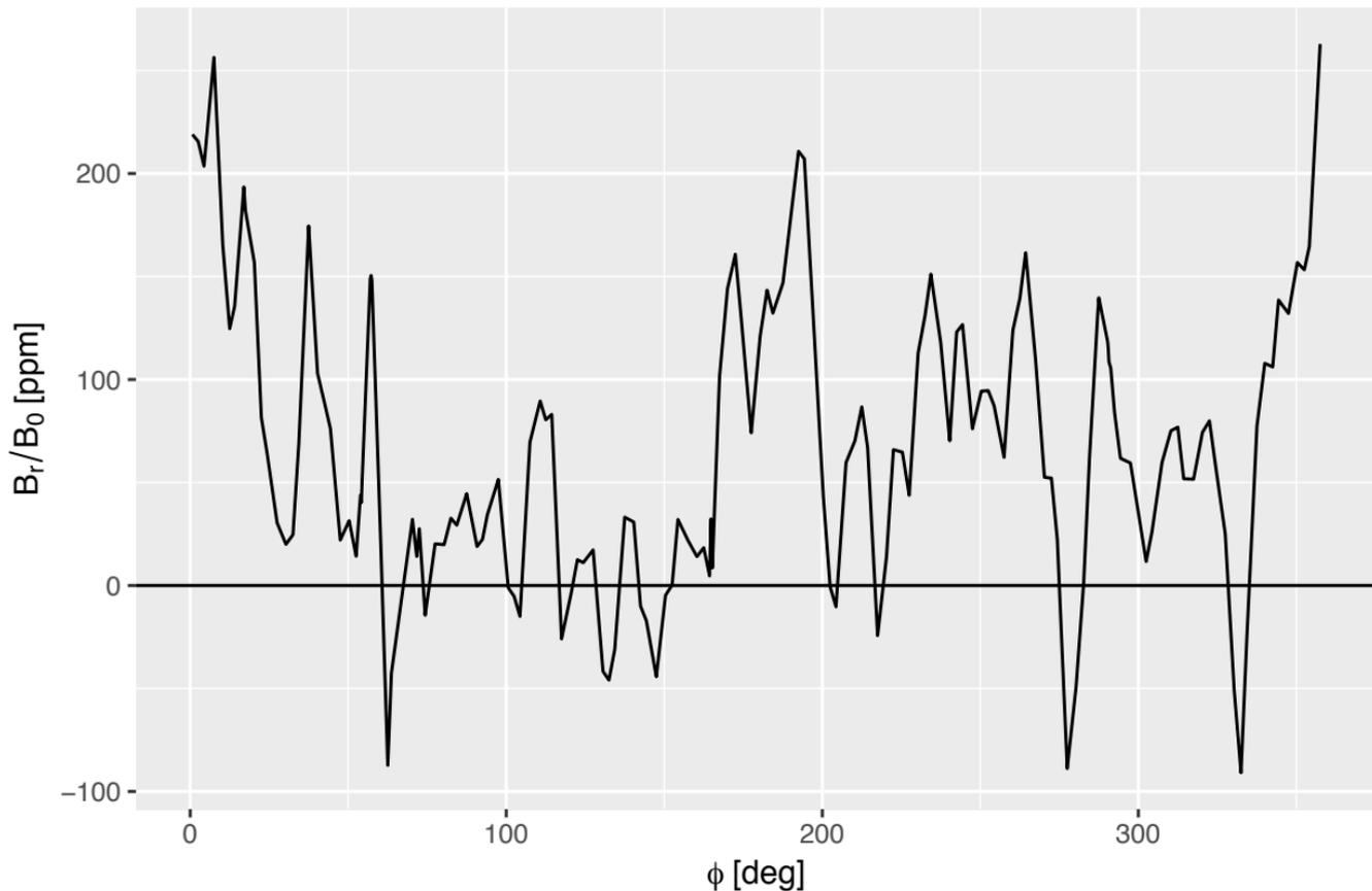
Surface coils have been tweaked to reduce the  $\langle y \rangle$  around the ring. To simulate, we take the radial data from 2016 *minus* 35 ppm, according to most recent shimming.
