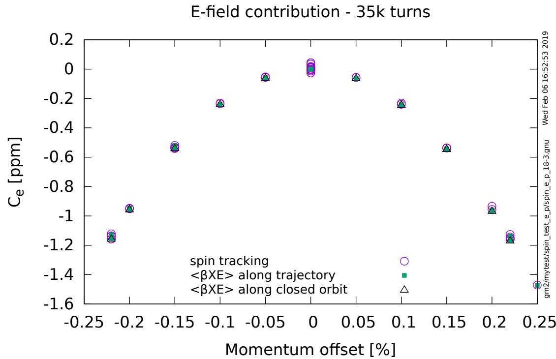
$\langle \beta \times \mathbf{E} \rangle$  along the trajectory is very nearly the same as  $\langle \beta \times \mathbf{E} \rangle$  along the closed orbit. (There is little dependence on betatron amplitude)
