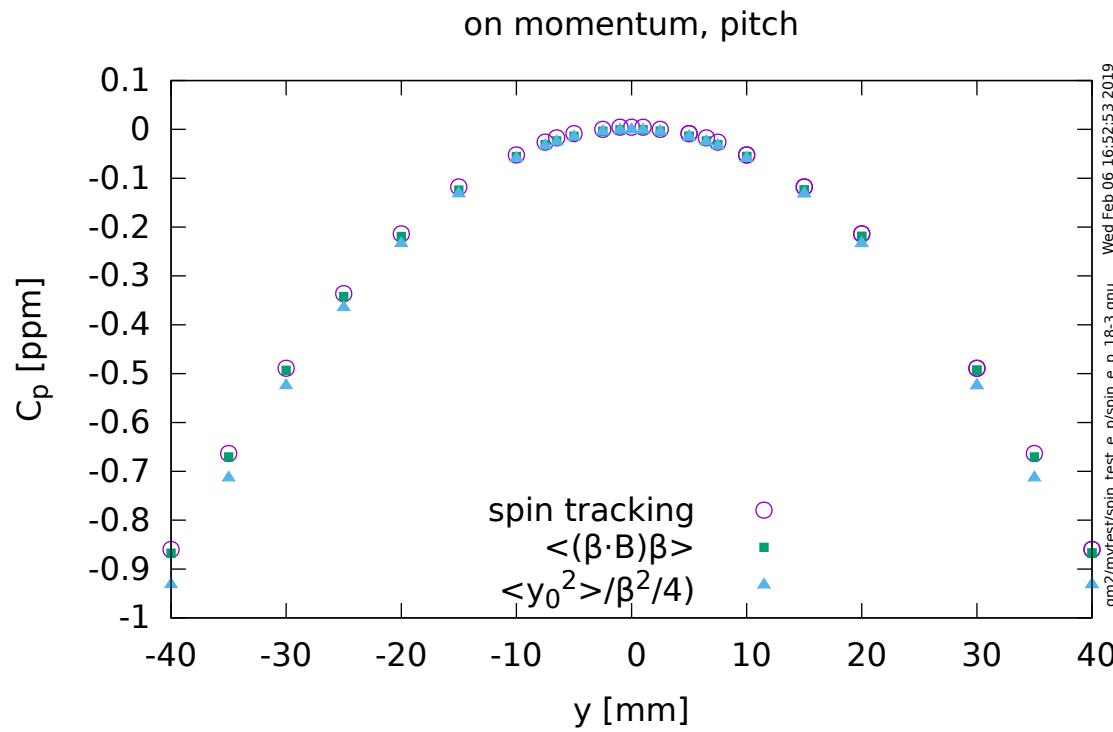
Vertical amplitude ( $y_0$ )/  $\beta_v$  is not a good measure of angle  $\psi$  at large amplitude
