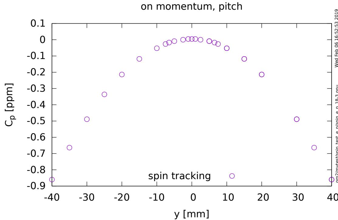
Pitch correction vs vertical amplitude
