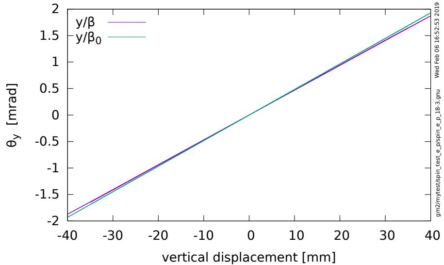
Quad nonlinearity  $\Rightarrow$  amplitude dependence of tune and  $\beta$
