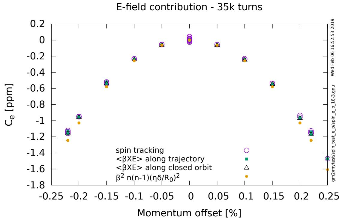
The calculation of the E-field correction that assumes quad linearity, *overestimates* the effect at large momentum offset (where E-field does not increase linearly with displacement)
