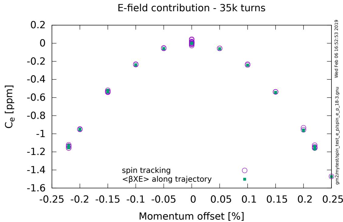
Efield correction computed with spin tracking in good agreement with correction based on  $\langle \beta \times \mathbf{E} \rangle$
