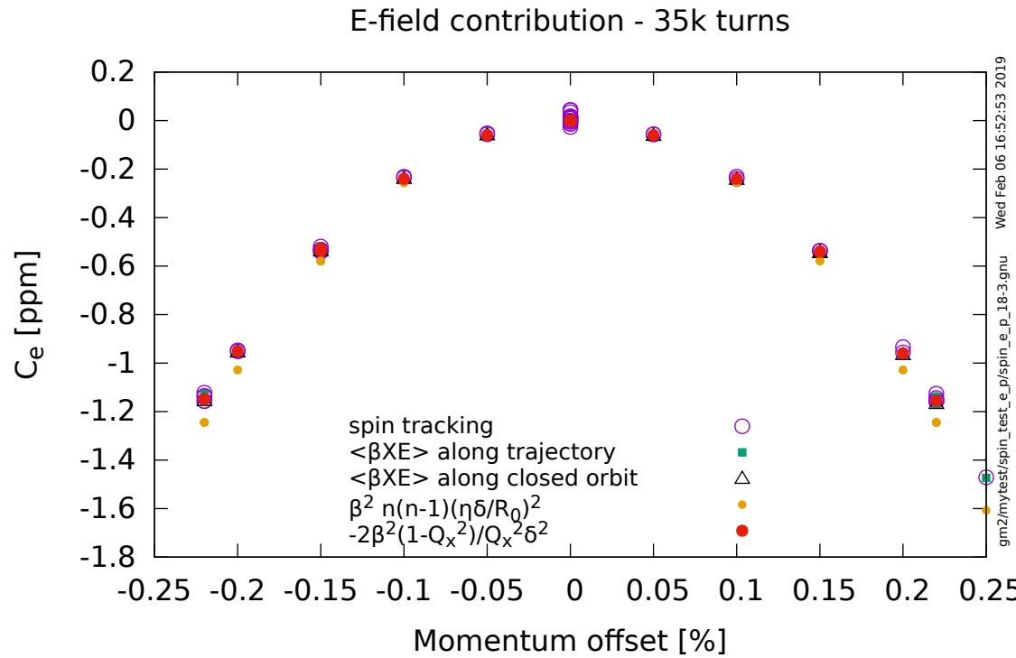
Replace  $n$ ,  $R_0$  and  $\eta$  with  $Q_x$  and measure  $Q_x$  for each momentum  $\Rightarrow C_e = -2\beta^2 \frac{(1 - Q_x)^2}{Q_x^2} \delta^2$
