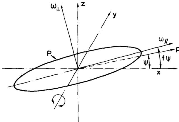
Fig. 1. Axes  $xyz$  rotating about  $z$  so that the momentum vector  $p$  lies always in the  $xz$ -plane. Owing to pitch oscillations the pitch angle  $\psi$  between  $p$  and the  $x$ -axis is varying. The spin angle is determined in the plane  $P$  (inclined at angle  $f\psi$  to the  $x$ -axis) because a spin in this plane moves into the  $xy$ -plane when  $\psi$  passes through zero.
