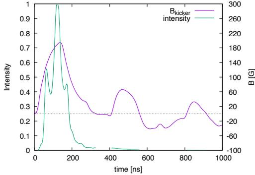
FIG. 2: The muon pulse (Run 1 T0 bunch 1) extends nearly 200 ns. The kicker pulse (Run 1 magnetometer measurement) is the purple curve. The peak of the kicker pulse is scaled to 204 G, typical in Run 1.
