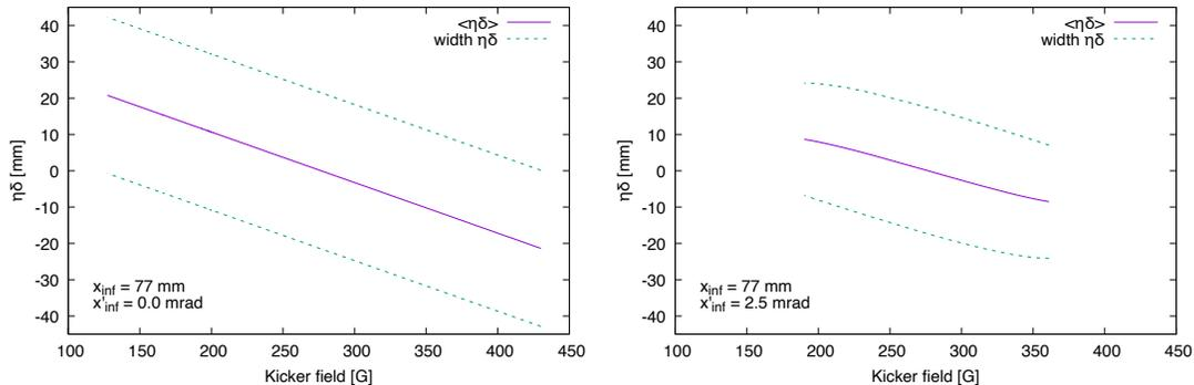
FIG. 1: Momentum acceptance as a function of kicker field, assuming  $x'_{inf} = 0$  (left) and  $x'_{inf} = 2.5$  mrad (right). All particle momenta between the dashed lines are stored. The solid line corresponds to the particle momentum (radial offset) that is kicked onto its closed orbit. The other momenta in the slice oscillate about their respective closed orbits with finite betatron amplitude. Note that the injection angle  $x'_{inf}$  reduces the momentum acceptance.
