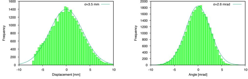
FIG. 7: Displacement(left) with respect to the center of the inflector aperture ( $x_{inf} = 77\text{mm}$ ) and angle of the trajectory at the inflector exit as determined by simulation. Both distributions are roughly gaussian. The overlaid Gaussian curves have widths  $\sigma_d \sim 3.5\text{mm}$  and  $\sigma_\theta \sim 2.6\text{ mrad}$  respectively.
