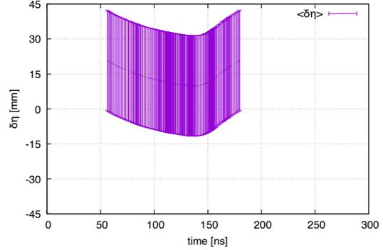
FIG. 3: The threshold kick angle for capture is  $\theta_k = (x_{inf} - A)/\beta = 4.5$  mrad  $\rightarrow$  122 G. The width of the range of captured momenta (the length of the error bar) is  $A/\eta$ . The midpoint of the range is  $\langle\eta\delta\rangle = \frac{1}{2}(x_{inf} - \theta_k\beta)$ . (The injection angle  $x'_{inf} = 0$ .)
