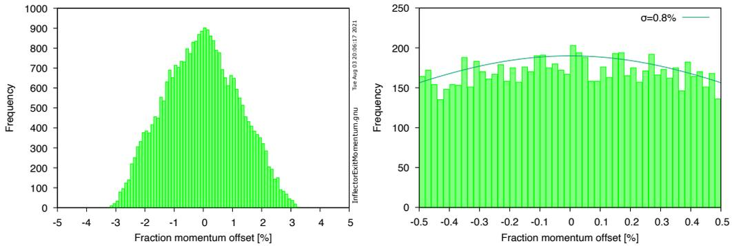
FIG. 4: Momentum distribution of all muons exiting the inflector (left). And those for which there are stable closed orbits in the storage ring (right). The shape of the distribution in the storable range corresponds (roughly) to a gaussian with  $\sigma = 0.8\%$ .
