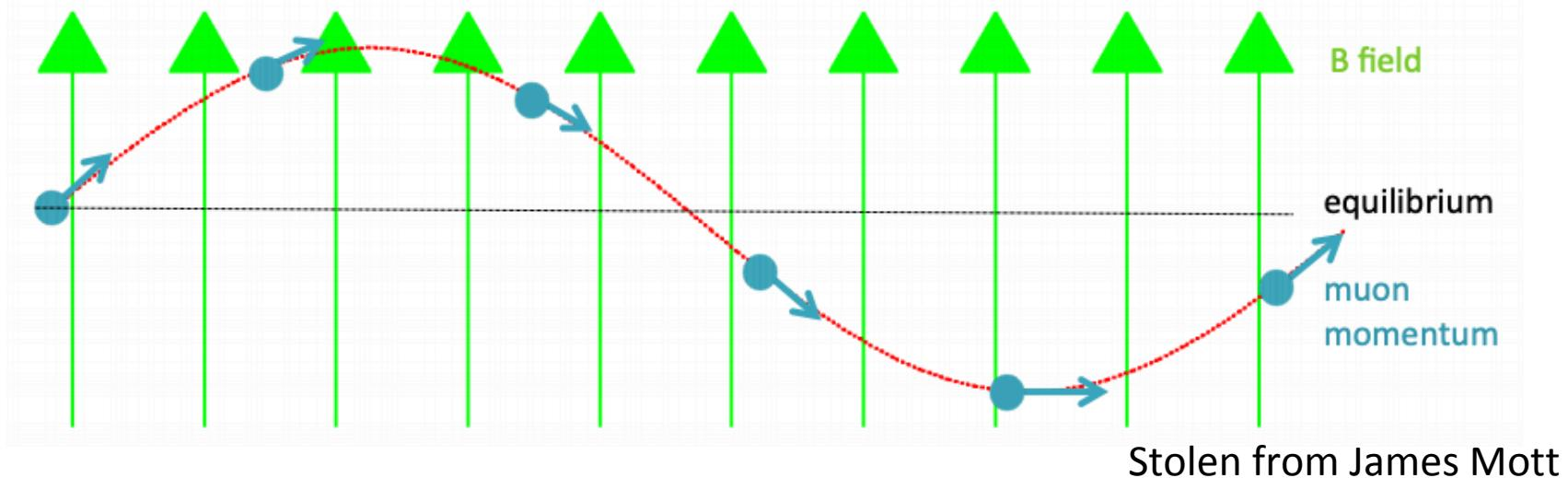
Precession in a single revolution is independent of vertical oscillation
