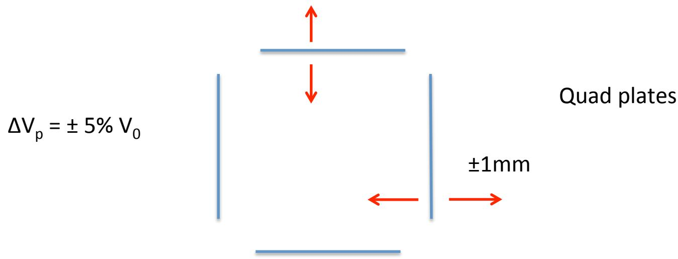
There are  $2^4$  combinations of displacement errors. Two for each plate and 4 plates
