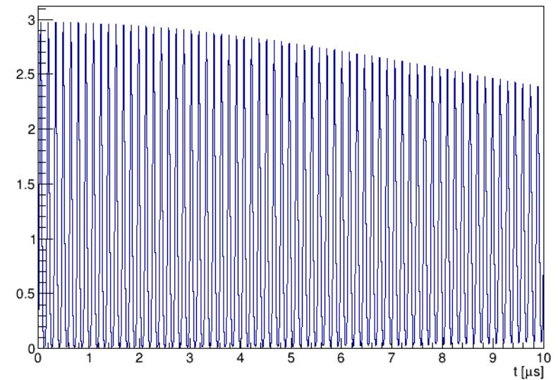
At  $t = 0$ , beam is maximally bunched. As  $t \rightarrow \infty$ , muons distributed uniformly around ring
