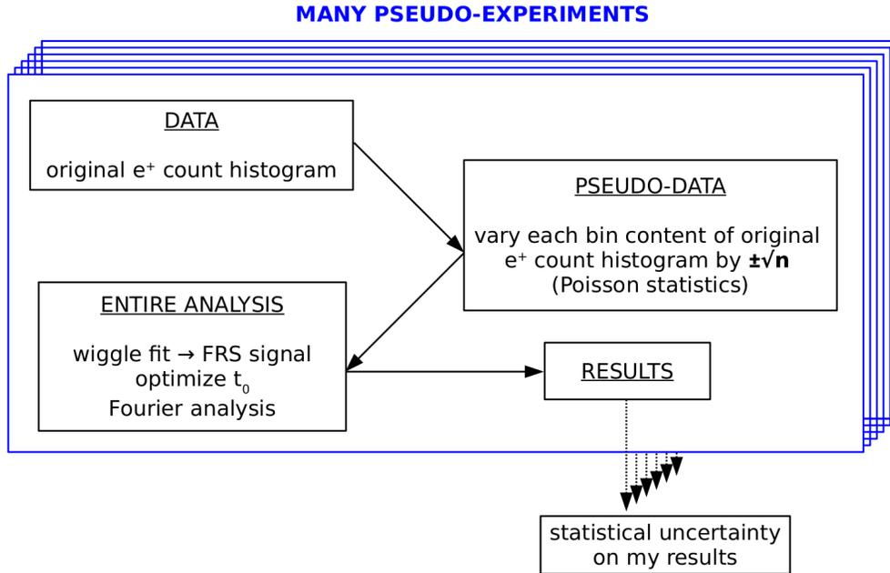
Figure 15: Diagram of the procedure for estimating the statistical uncertainty on the fast rotation results.
