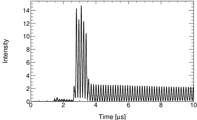
Figure 4: Fast rotation signal as a function of time as seen by all the calorimeters combined in the Run-1 EndGame dataset, between 0 – 10  $\mu\text{s}$  after beam injection. The time interval is 1 ns.
